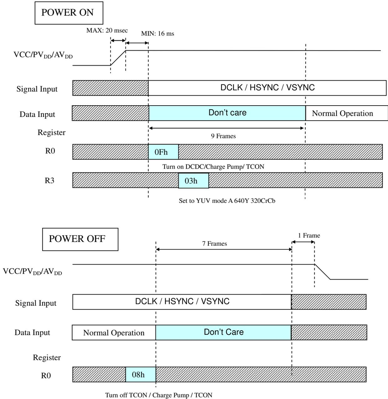
**7. Recommend YUV mode A 720Y 360CrCb (27 MHz) power on/off setting**
