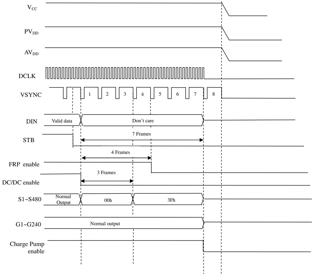
Note 1: External signal: V<sub>CC</sub>, PV<sub>DD</sub>, AV<sub>DD</sub>, DCLK, VSYNC, DIN (D0 ~ D7), STB (By register)
