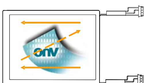
Fig. 2 Reverse scan (Pin4, REV = High)
