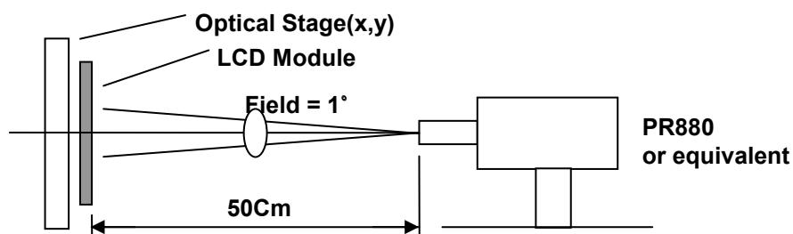
[Figure 9] Optical characteristic measurement equipment and method
