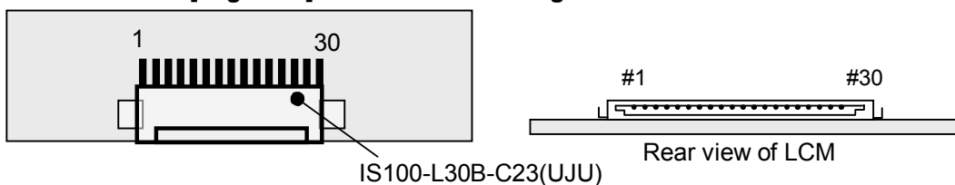
[ Figure 4 ] User Connector diagram
